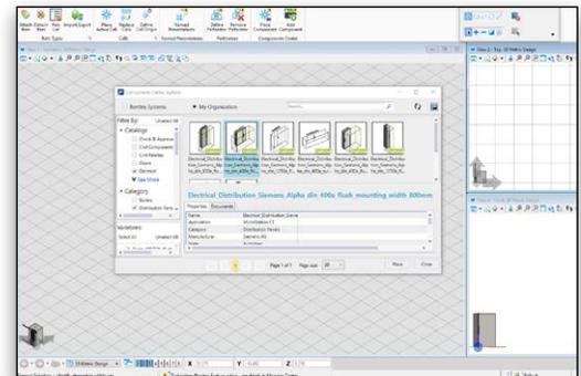
*Components Center can be accessed via plugins for Bentley products like MicroStation.*
